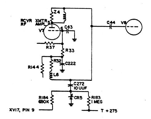
Figure 1. Schematic Diagram, After Modification
